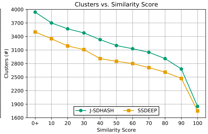
Figure 2: Absolute Number of Clusters per Similarity Threshold for the two similarity hashing functions.
